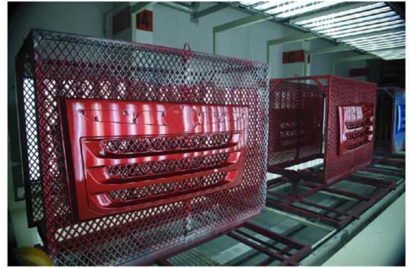
前围喷涂 Cabin Front Painting
