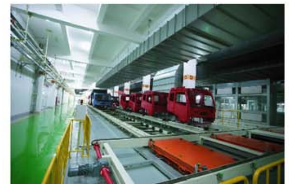
车身转运 Cabin Convey
