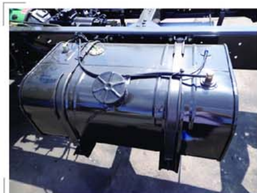
铁油箱 Steel Fuel Tank
