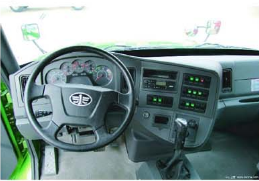
环绕仪表台&CAN仪表&四幅方向盘 Surrounding Dashboard & CAN Instrument & Four-spoke Steering Wheel
