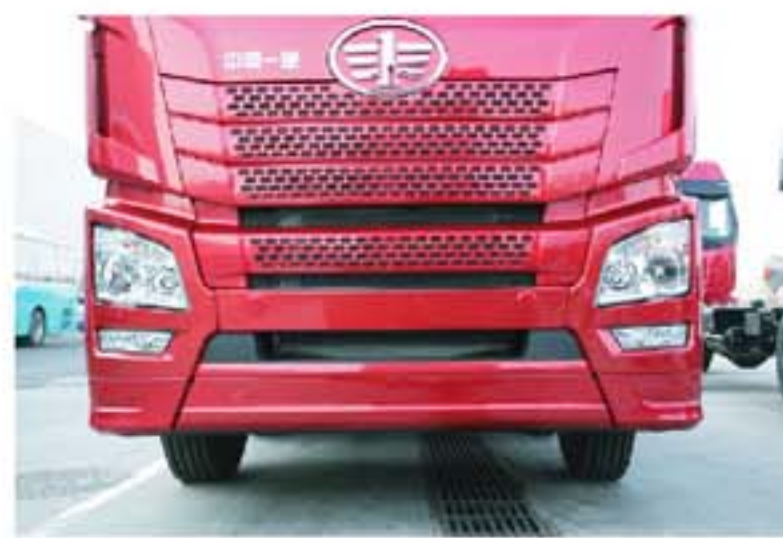
三段分体式金属保险杠&LED日间行车灯 Three Pieces Metal Bumper & LED Daytime Lights
