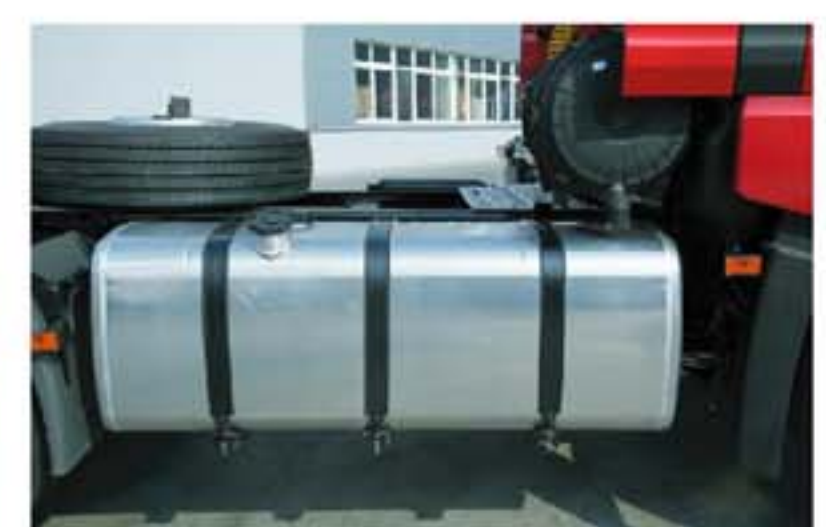
800L铝油箱 800L Aluminum Fuel Tank
